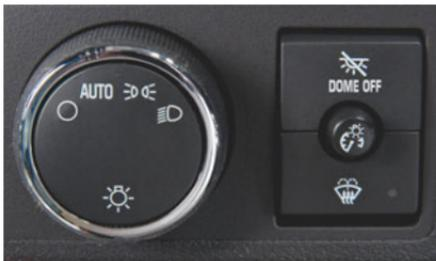
The exterior lamp control knob on the left side of the instrument panel can be rotated to the following positions:
