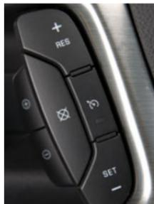
– **SET (Set)**: Press this button to set a speed, or to decrease the speed if the system is active. When the cruise control speed is set, the cruise control light will illuminate on the instrument panel cluster.
