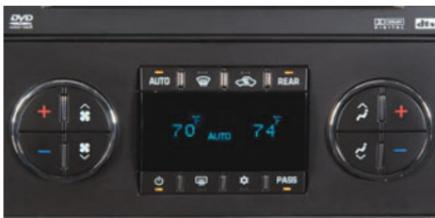
The automatic climate control system maintains the desired individual temperature for the driver and front seat passenger. The system adjusts the airflow mode, fan speed, air conditioning and recirculation functions to reach the set temperature(s) as quickly as possible.
