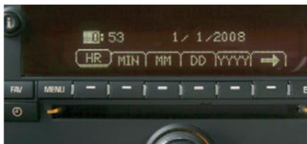
3. Press the pushbutton under any of the labels to be changed.
