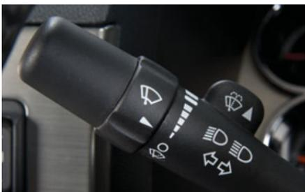
The following windshield wiper controls are located on the multifunction lever on the left side of the steering column:
