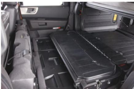
Reverse these steps to raise the Midgate. The Midgate must be fully latched before the window can be raised.
